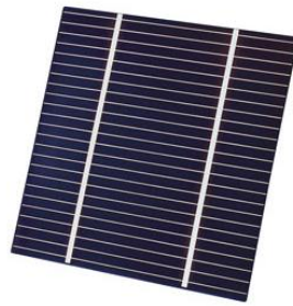
Figure 18. Mono-crystalline Silicon cell of 50x50 mm with printed metallic front contacts.
