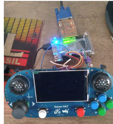
Fig. 9. CoLenda prototype on a DE0-Nano FPGA platform.
