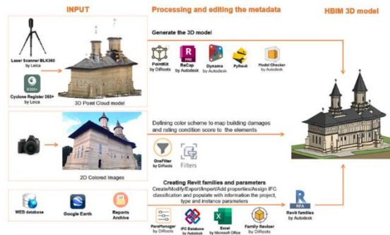
Fig. 2. Proposed methodology - Stages to process and edit the input data and generate the Revit model.
