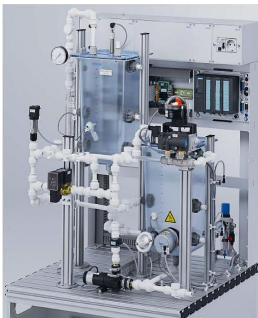
Fig. 2 MPS®PA Compact Workstation FESTO
