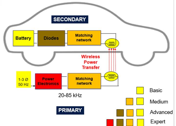
Figure 1. Relationship between the levels of the gamification technique and the components of the EV wireless charger that are acquired in each level.
