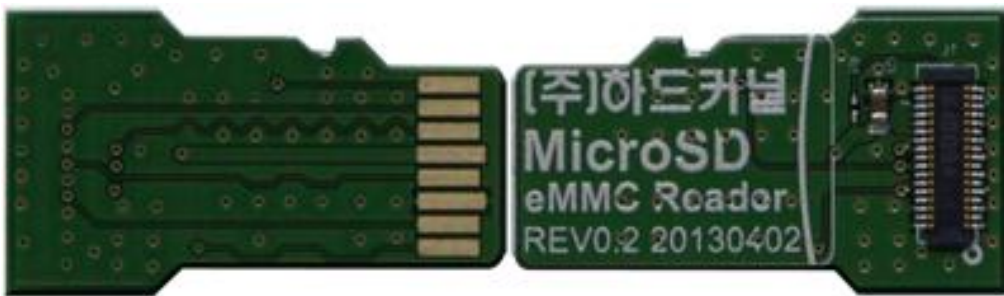
Figura 6.2. 16GB eMMC V5.0 to MicroSD Adapter
