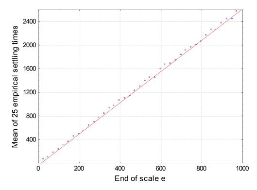
Figure 4.11. End of scale vs. settling time.
