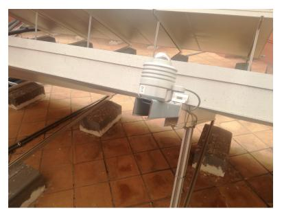
Figure 13: Pyranometer installed in the hotel's rooftop.
