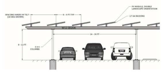
Figure 2: Inter-row distance in the solar carport to be kept [5].
