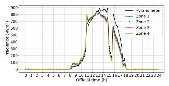
Figure 15: Incident irradiance values measured on the pyranometer and those calculated for each solar carport zones on the 21st of December after the correction factors are applied .
