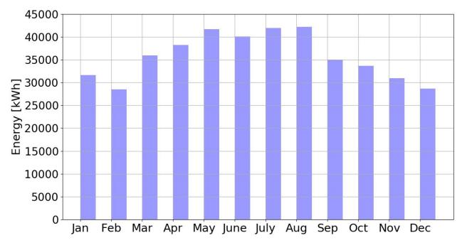
Figure 17: Energy delivered by the PV system in each month of the first full year of operation.
