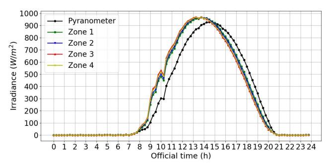
Figure 14: Incident irradiance values measured on the pyranometer and those calculated for each solar carport zones on the 21st of June after the correction factors are applied.
