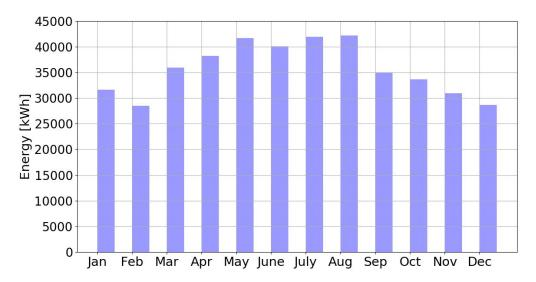
Figure 5: Energy delivered by the PV system in each month of the first full year of operation.
