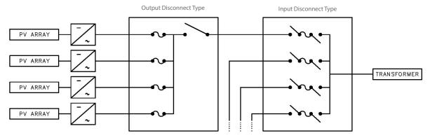
Secondary AC Combiners are typical for sites where further agreggation of AC Combiners is needed.
