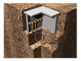
Figure 7: Earthing installation [2].
