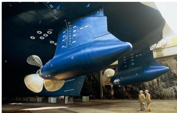
Foto 24: Hélice Azimutal. Fuente: [http://www.motorship.com/\\_\\_\\_data/assets/image/0009/726561/AZIPOD6\\_hi-2.jpg](http://www.motorship.com/___data/assets/image/0009/726561/AZIPOD6_hi-2.jpg)
