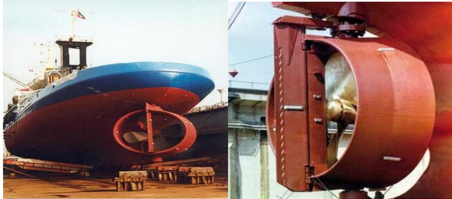
Foto 17 y foto 18: Timón-Tobera Kort. Fuente: <http://www.fairplay-towage.com/files/fairplay-ix-dock-kort-duese.jpg> [http://img.nauticexpo.es/images\\_ne/photo-g/tobera-helices-buques-30793-178565.jpg](http://img.nauticexpo.es/images_ne/photo-g/tobera-helices-buques-30793-178565.jpg)
