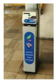
To use the machine, lay your ticket with the front side face down, magnetic stripe facing up, on the black plastic area and slide the ticket to the left. Wait for the machine to make a loud stamping noise after which your ticket should be punched and validated. Orientation of the ticket, besides magnetic strip facing up, doesn't matter.
