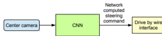
Figure 3: The trained network is used to generate steering commands from a single front-facing center camera.
