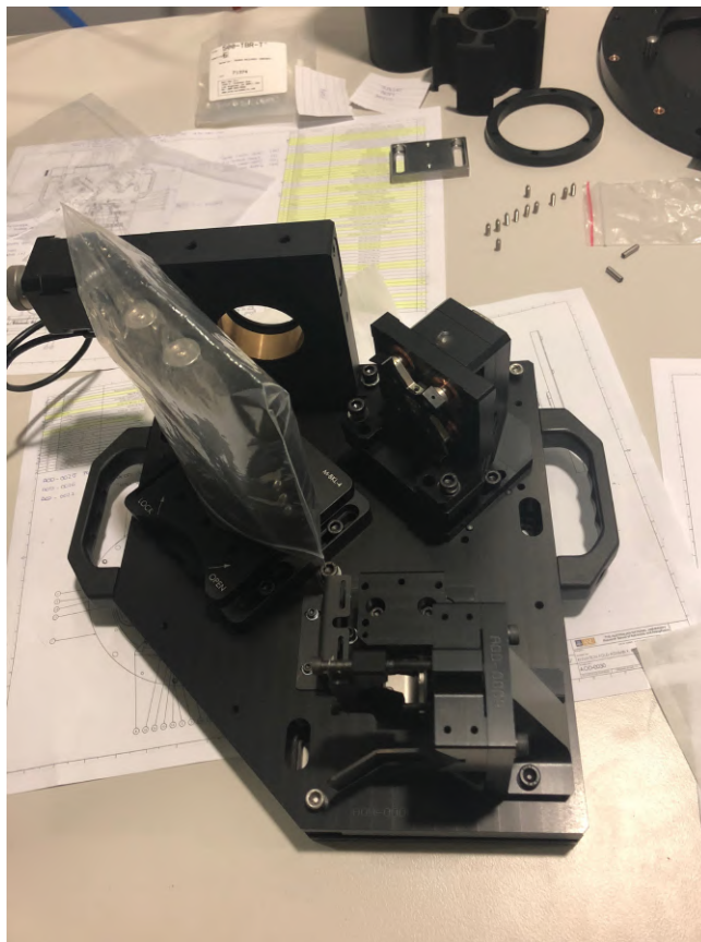
FIGURE B.7: BTO base plate which allows the attachment and independent alignment of the BEU, BCM, LFM and HWP units.
