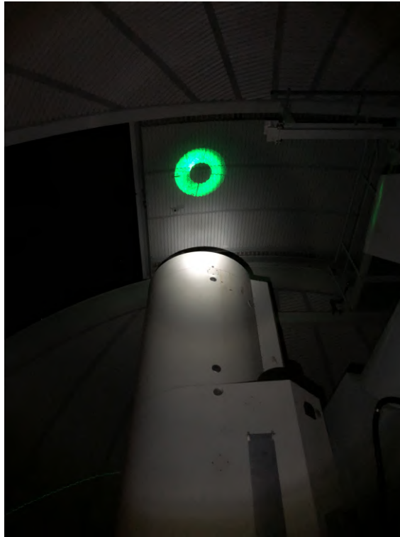
FIGURE 7.5: Above, the ring-shaped generation with the axicon during alignment tasks; below, the laser ring at the OGS dome.
