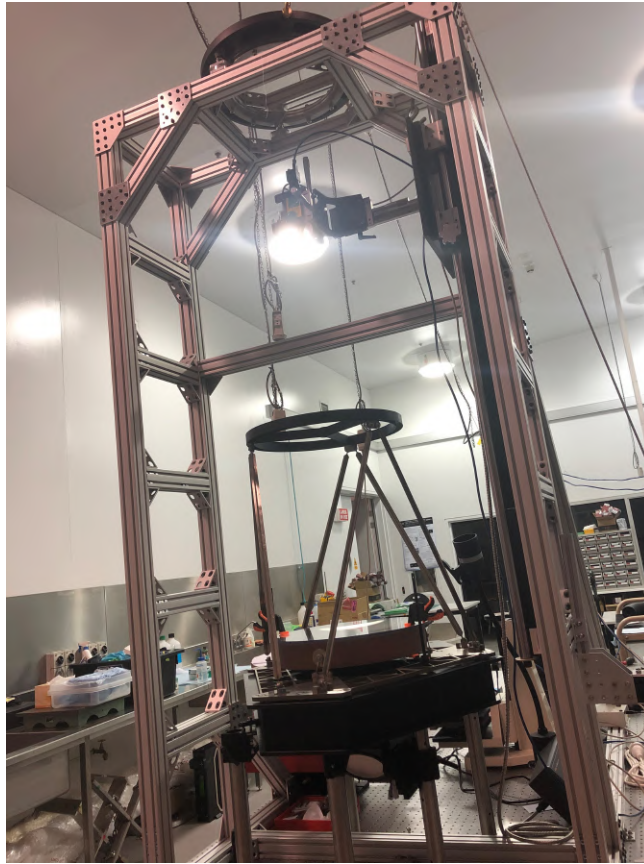
FIGURE B.23: The LLT is mounted on the shown structure for alignment purposes.
