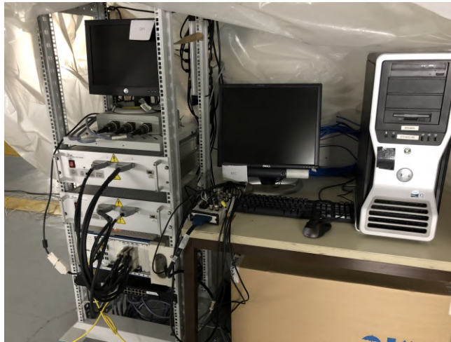
FIGURE 7.17: UWCS Control System: from left to right, electronics cabinet with CILAS control modules on top (junction box and two signal amplifiers), National Instruments PXI-E and Ethernet switch below, and RTC PC.
