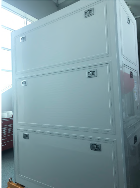
FIGURE B.5: Guide Star Laser Enclosure. The Beam Transfer Optics will be mounted on the middle bench, whereas the upper and lower breadboards are assigned to the GSLP and the OPSL subsystems.
