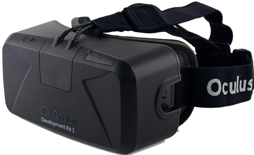
Figura 11: HMD de Oculus Rift Development Kit 2.
