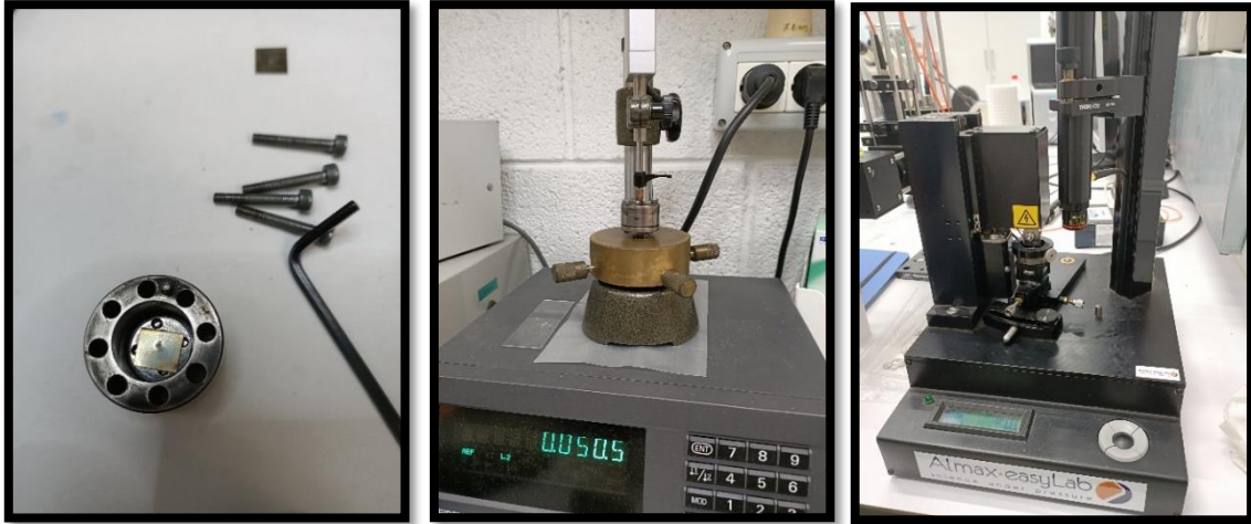
Fig. 10. (Left) Diamond anvil cell with a gasket inside. (Centre) Heidenhain ND221B length gauge. (Right) Almax EasyLab Electrical Discharge Machining.
