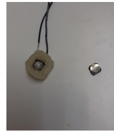
(b) Dissected and welded buzzer
