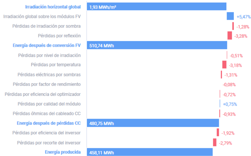
figure 9: annual production of the photovoltaic installation and loss factor
