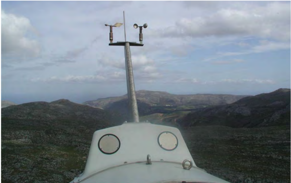
Figure 4.36: Example of wind measuring instruments on a wind turbine
