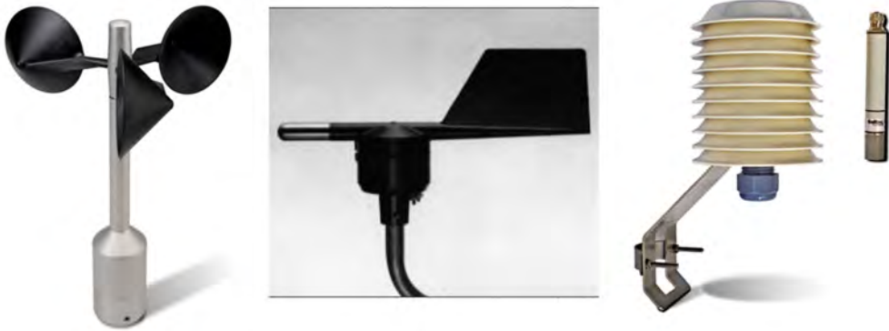
Figure 4.33: Beginning from the left, the figure shows anemometer, weather vane and thermometer
