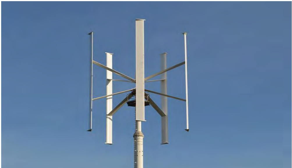
Figure 4.28: An image of a vertical axis wind turbine 7
