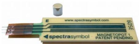
Figura 6. Sensor magnetopot.
