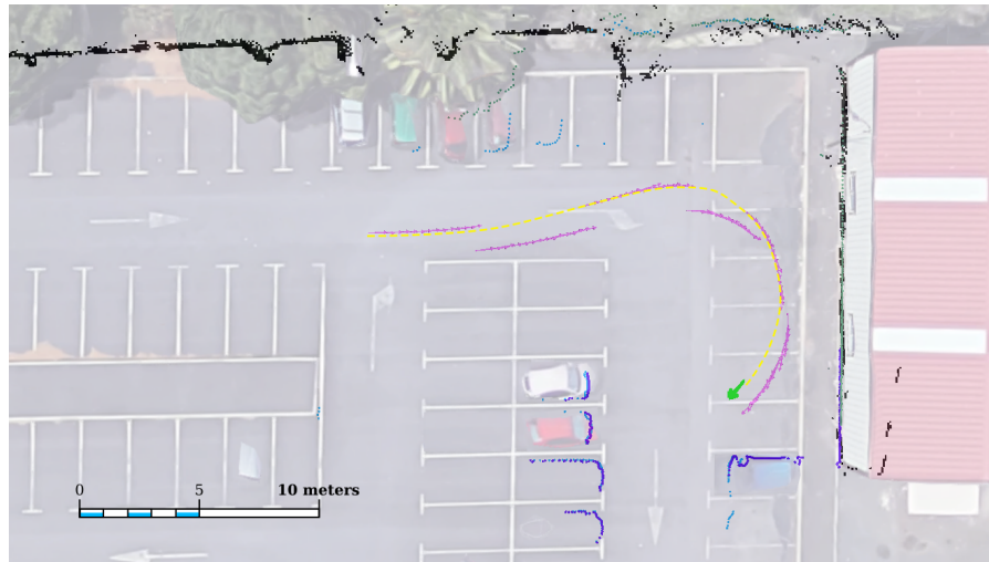
Figure 2.1 Localization with particle filters. Green arrows: set of particles from the localization hypotheses estimated by the PF; magenta arrows: GPS readings; green, blue and purple dots: features from LiDAR scans; yellow dashed line: ground truth of the trajectory; black: obstacles represented in the map.
