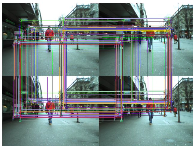
Figure 6. Common points between frames t and t - 1 in the matching cycle.
