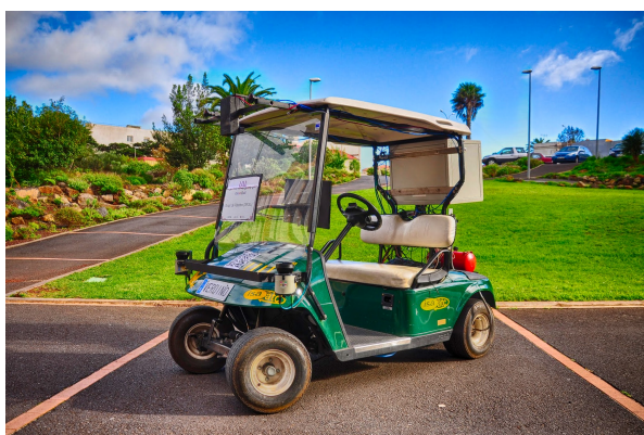
Figure 2. The algorithm is intended for the Verdino prototype, designed to travel in pedestrian environments.
