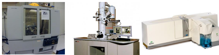
Fig. 3.4. (left) PANalytical X'Pert PRO diffractometer (Bragg-Brentano geometry), (center) JEOL JEM 2100 and (right) Mastersizer 2000/E equipments.
