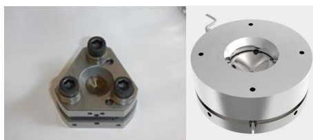
Fig. 3.11. (left) Merrill-Basset type DAC for XRD experiments and (right) membrane-type DAC for Raman scattering and luminescence experiments.
