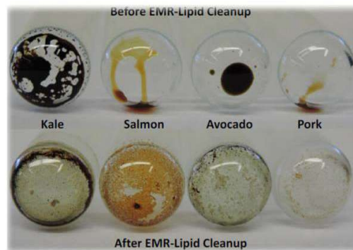
Figure I.5.- Image of non-evaporated co-extracts from different matrices before and after EMR-Lipid clean-up. Reprinted from [247] with permission from Elsevier.
