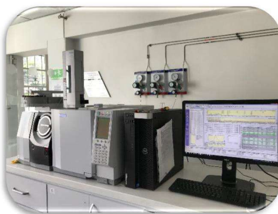
Figure III.1.- Photograph of the GC-QqQ-MS/MS system used in this PhD Thesis.
