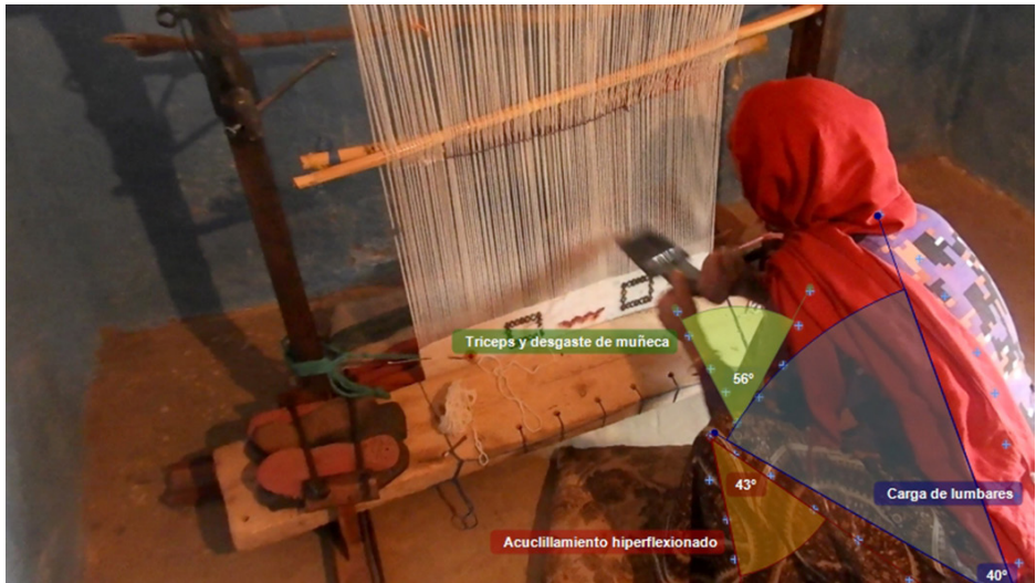
Figure 6. Biomechanical analysis of the video taken of a woman weaving on a horizontal loom in the Tislit douar.
