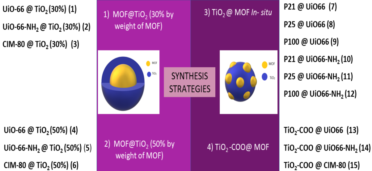
Fig S3. The scheme of the fabrication and synthesis of 1-15 composites
