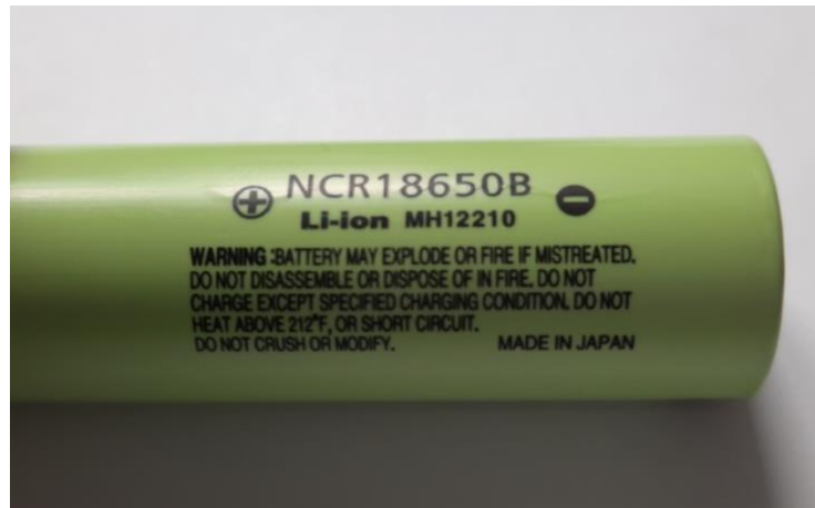
Figura 55: Pila PANASONIC NCR18650B
