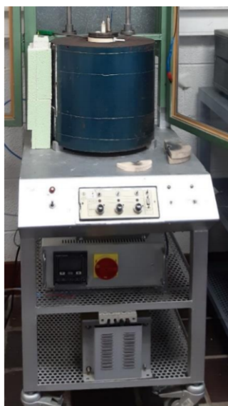
Fig. 13: Oven used to heat the sample during impedance spectroscopy testing.
