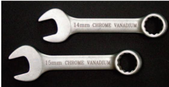
*Low alloy chrome-molybdenum and chrome-vanadium steels are used for high-quality tools, bike frames, and automobile engine and transmission components.*
