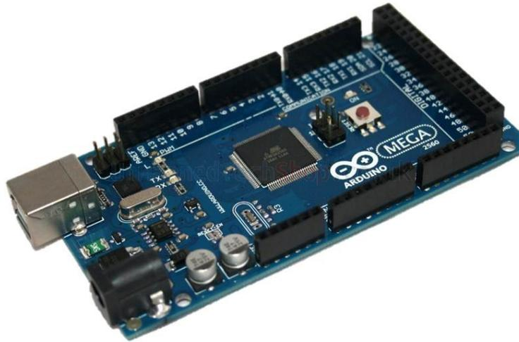
**Figura 3.1:** Arduino Mega 2560
