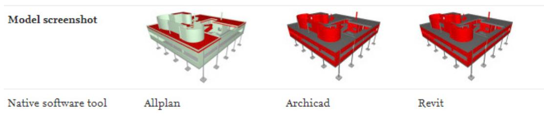
**Figura 12.** Captura de pantalla de los modelos exportados a IFC. Assessment of model-based data exchange between architectural design and structural analysis. Goran Sibenik, Iva Kovacic, 2020
