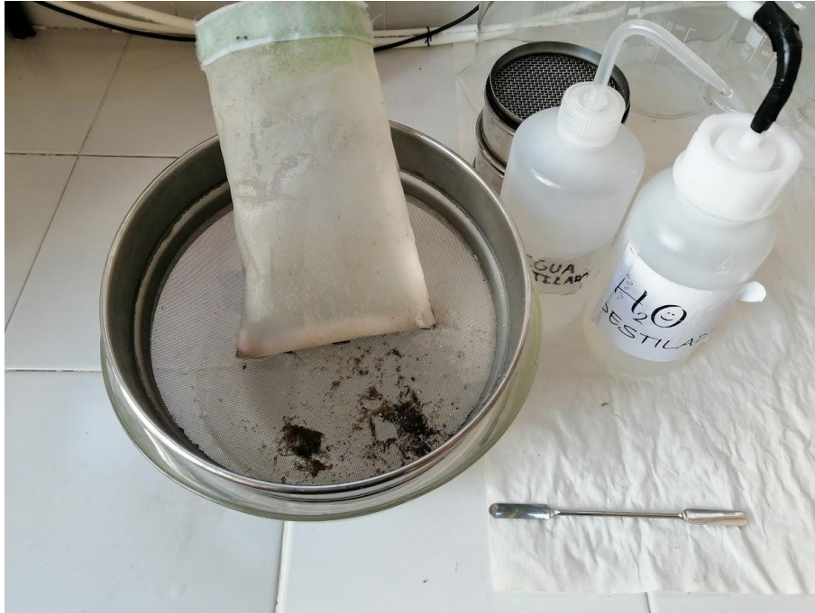
Figure 4. The first step in the laboratory work. It can be seen the collector bag inverted, distilled water and the 315 \mu\text{m} sieve.
