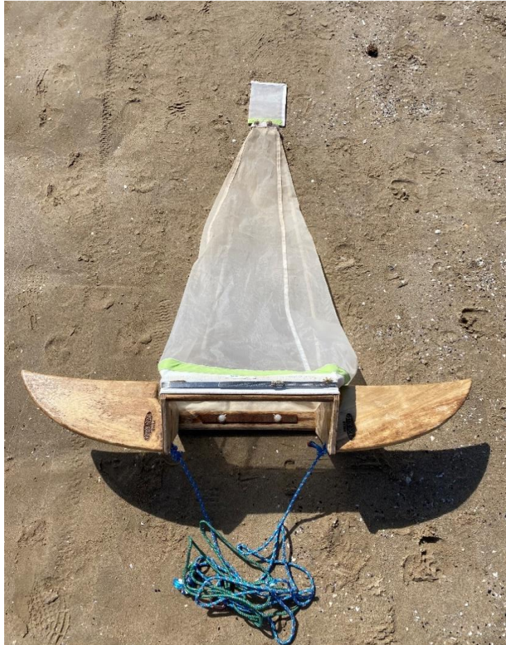
Figure 2. Paddle-trawl used for samplings, with de 335 \mu m net, the collector bag and the 3 m rope.
