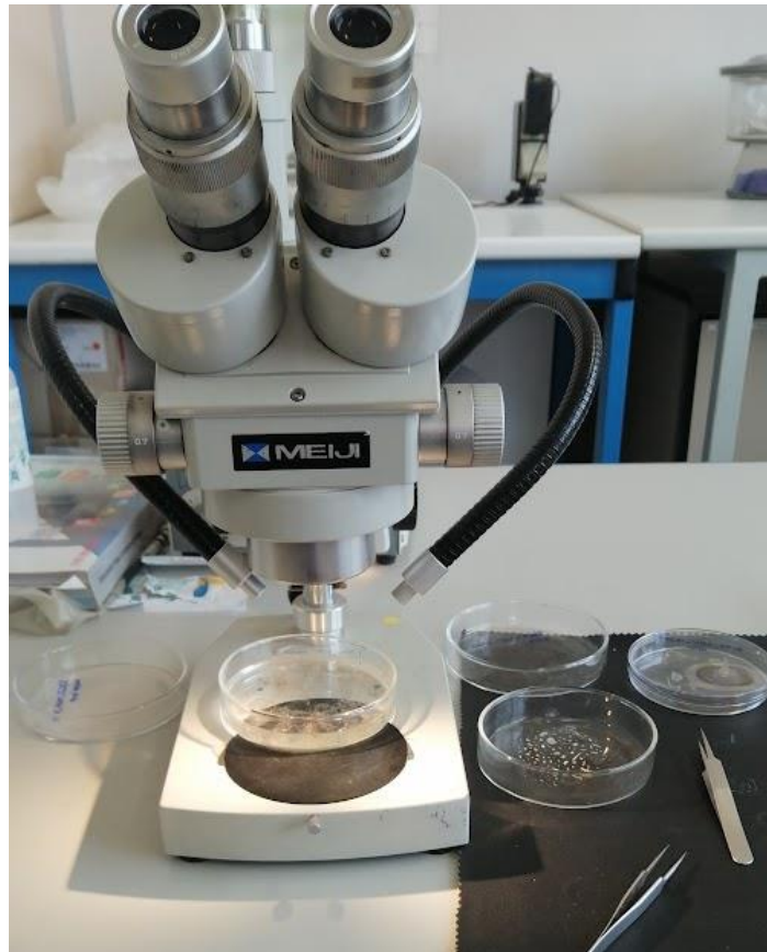
Figure 5. The stereo-microscope used in the third step in the laboratory work. Petri dishes with non processed plastics, the new dry Petri dish and the stainless-steel tweezers used.
