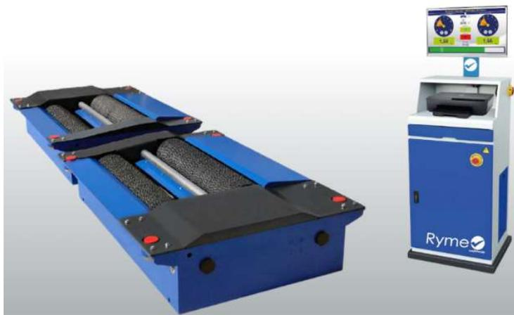
Figura 26. Frenómetro. Fuente: [https://www.ryme.com/wp-content/uploads/Descargas/Catalogo-Ryme-2021-%20ESP\\_compressed.pdf](https://www.ryme.com/wp-content/uploads/Descargas/Catalogo-Ryme-2021-%20ESP_compressed.pdf)
