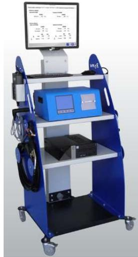
**Figura 24. Analizador de gases. Fuente: [https://www.ryme.com/wp-content/uploads/Descargas/Catalogo-Ryme-2021-%20ESP\\_compressed.pdf](https://www.ryme.com/wp-content/uploads/Descargas/Catalogo-Ryme-2021-%20ESP_compressed.pdf)**
