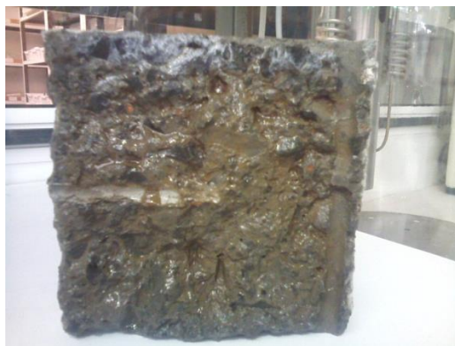
Figure 6. Chloride penetration profile revealed. The chloride penetration front can be seen in the upper part of the broken sample.
