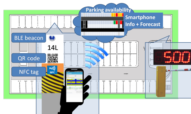
Figure 3. Low-cost indoor parking system.
