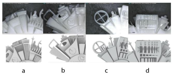
**Figure 4.** Images of the print test (Ameralabs Town) made at  $30 \times$ . (a) Surface textures, (b) "Alternating deepening plates" test, (c) "Cross-shaped bridges" test, (d) Minimum width of the opening" and "Minimum Height of the opening" test.
