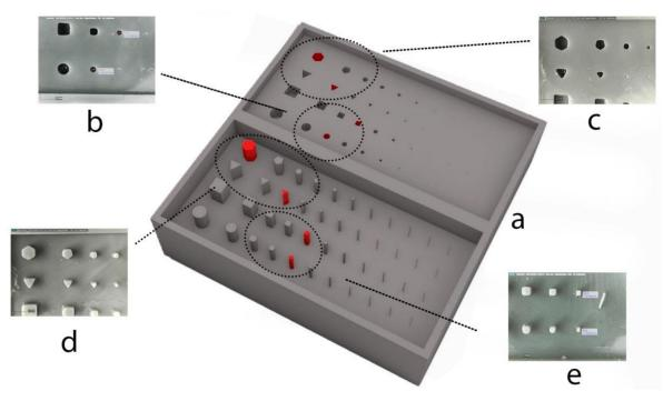
**Figure 5.** Calibration test results for XY axes. made at  $25 \times$ . (a) Designed test, (b) best result for square and circular negative shapes (c) best results in triangular and hexagonal negative shapes, (d) best results for hexagonal and triangular positive shapes, (e) best results for square and circular positive shapes.
