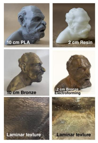
Figure 1. Examples of figures made by PLA (polylactic acid) and resin molds.
