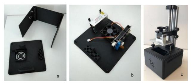
Figure 3. 3D printed parts. (a) Case, (b) Base, (c) All the printed parts.
