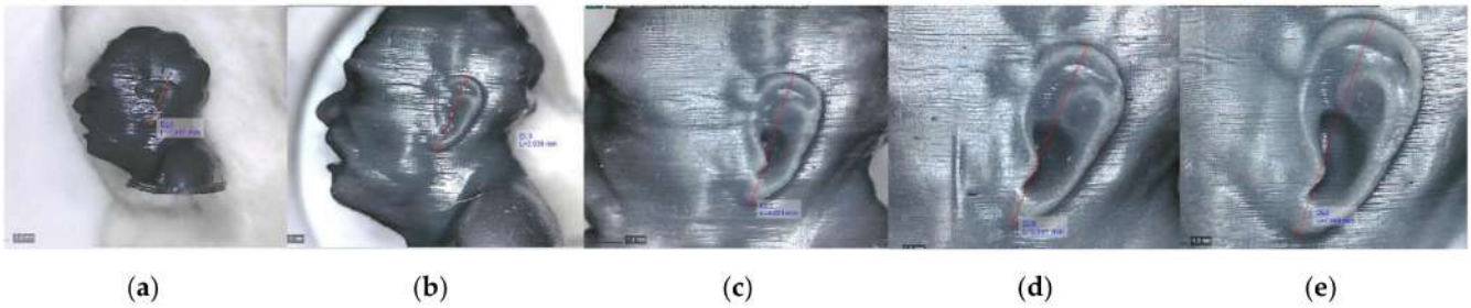
Figure 7. From left to right (a–e), ear detail from pieces of 5 mm, 10 mm, 15 mm, 20 mm, and 30 mm in height.
