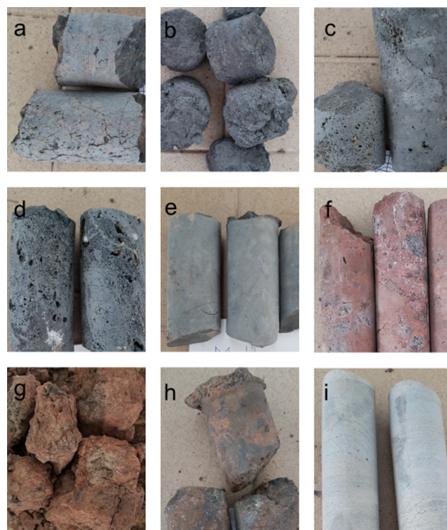
Fig. 1. Lithotypes. The identified lithotypes were: (a) aphanitic massive basalt, (b) altered and highly altered aphanitic massive basalt, (c) vacuolar aphanitic basalt (vacuole < 0.05 mm), (d) vacuolar aphanitic basalt (vacuole < 0.3 mm), (e) phonolite, (f) red colour ignimbrite (vacuolar basaltic fragments), (g) highly altered red colour ignimbrite (vacuolar basaltic fragments), (h) agglomerate basaltic materials, (i) massive and vacuolar plagioclase basalt (Füster et al., 1969). (For interpretation of the references to colour in this figure legend, the reader is referred to the web version of this article.)
