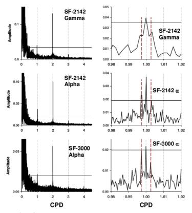
Fig. 8. Spectra (FFT) of de-trended time series at sites SF-2142 and SF-3000. Left column the daily variation band. Right column detail around S1 periodicity, demonstrating the occurrence of sidebands at the specific frequencies of LSb and USb (shown as vertical lines).
