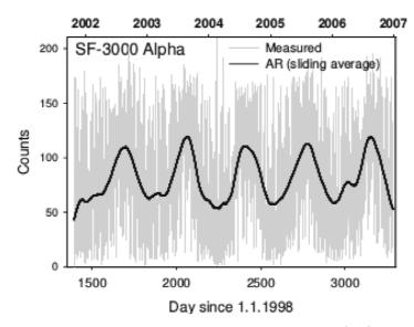
Fig. 5. SF-3000. Measured alpha signal and the annual radon (AR) signal applied for detrending the time series (Day 0 = 1.1.1998).
