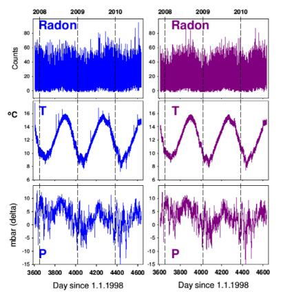
Fig. 3. Day-time (left column) and night-time (right column) time series of radon, temperature and pressure, at MM-0 (Day 0 = 1.1.1998).
