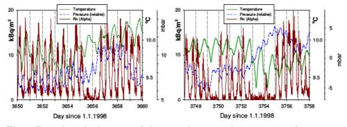
Fig. 2. Example 10-day long interval showing radon, atmospheric pressure and temperature variation patterns in MM-0 bunker (Day 0 = 1.1.1998). The variation of radon is dominated by two peaks per day.
