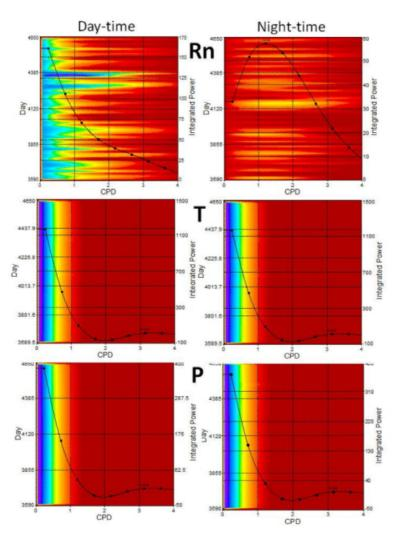
**Fig. 4.** Continuous Wavelet Transform spectral analysis of the time series shown in Fig. 3, presented as Time Integrated Power Spectral Density. The analysis is based on the Paul (complex) wavelet, with wavenumber order = 16. The curve (black) is the Time-Integral Squared Amplitude Power. Different day- and night-time patterns are obtained in the case of radon.
