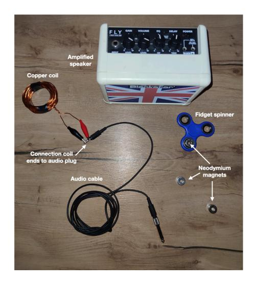
Figure 1. Picture showing all the components of the demonstration, including the setup of the connection between the coil and the audio cable.
