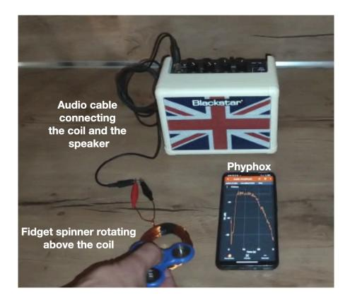
Figure 2. Snapshot of the demonstration, where the rotating spinner, with the magnets at the ends of the blades, is held in one hand above the coil. The gain and volume of the speaker are set to max, whereas the application phyphox is recording and plotting the amplitude of the sound, that is related to the voltage of the coil. Click on the figure to watch a video about the demonstration.
