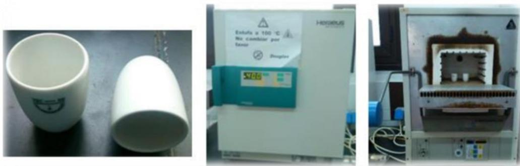
IMAGEN 2. CÁPSULAS PARA MUESTRAS, ESTUFA Y MUFLA
