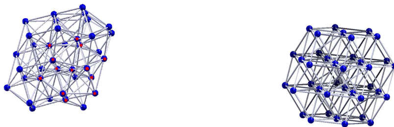
(a) Mackay Icosahedron structure for N = 37 (b) Truncated octahedron structure N = 38 . with the Mackay Icosahedron denoted by the red dots.
