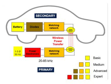
Figure 1. Relationship between the levels of the gamification technique and the components of the EV wireless charger that are acquired in each level.
