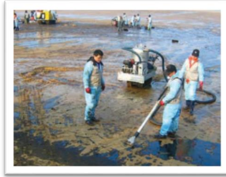
Ilustración 45 skimmer portátil; Fuente: http://www.itopf.com/knowledge-resources/documents-guides/document/tip-5-use-of-skimmers-in-oil-pollution-response/
