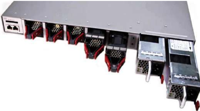
Figure 6. Redundant Fan and Power Supply
