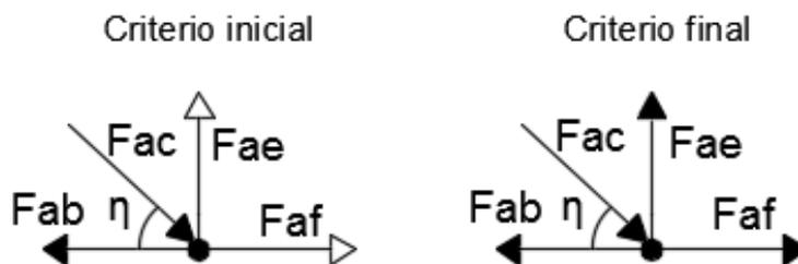
$$\Sigma F_x = F_{af} - F_{ab} + F_{ac} \cos \eta = 0 \longrightarrow F_{af} = 261,2718 \text{ KN}$$
